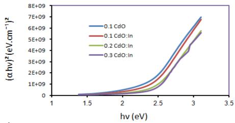
Fig. 5: The  $(\alpha hv)^2$  versus photon energy (hv) of various molar concentration for CdO and CdO:2%In films
