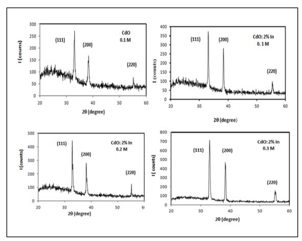
Fig. 1: The X ray diffraction (XRD) patterns of the prepared CdO and CdO:2%In films of different molar concentrations
