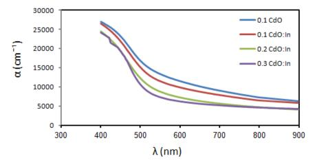
**Fig. 3:** Variation of optical absorption coefficient with wave length for various molar concentrations of CdO and CdO:2% In films
