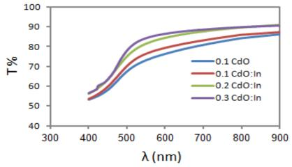
Fig. 2: Optical transmittance spectra of the CdO and CdO:2%In of different molarities films in the range of (400 - 900 nm)
