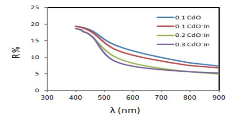
**Fig. 6:** Optical reflectance spectra of various molar concentration for CdO and CdO:2%In films The extinction coefficient of all films was calculated from equation (Benramdane, N., *et al.*, 1997; Ferro, R., *et al.*, 2000):
